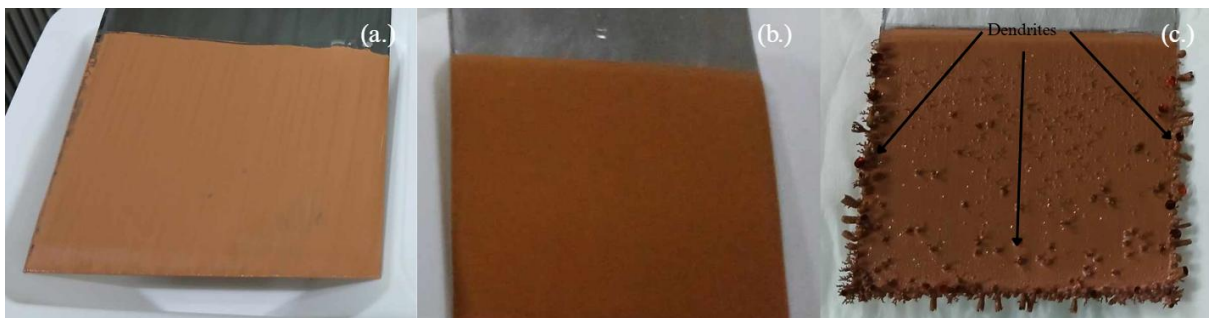
Figure 6. Electrorefining at 40 g/L Cu concentration at (a.) 50 A/m 2 , (b.) 100 A/m 2 , (c.) 150 A/m 2 without agitation
